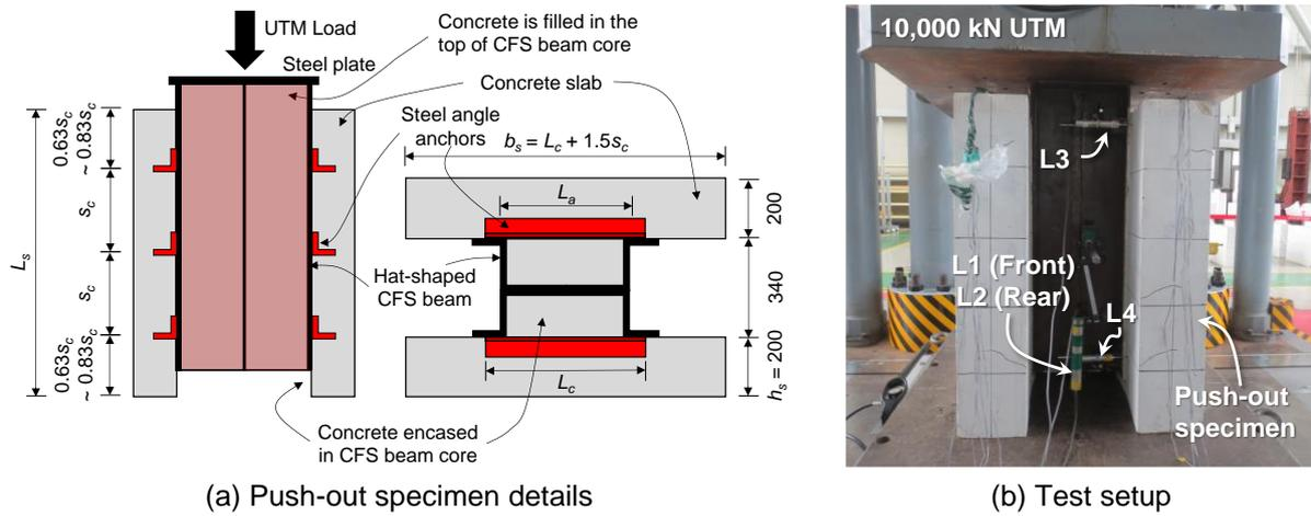
Fig. 1 Push-out specimen details and test setup
