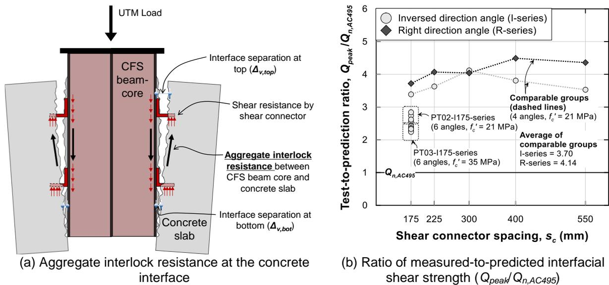
**Fig. 2** Interfacial shear strength evaluation of angle shear connectors welded to U-shaped steel beam
